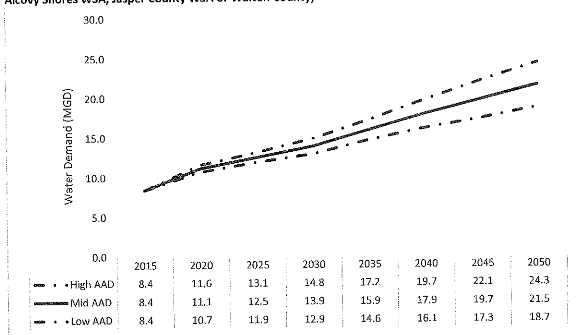
Figure 3.3: Annual Average Day Water Demand for Newton County (does not include demand for Alcovy Shores WSA, Jasper County WSA or Walton County)
